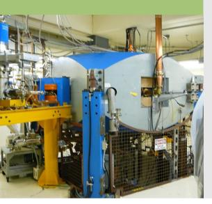
EBCO (now Advanced Cyclotron Systems Incorporated) constructs a prototype compact TR-13 cyclotron at TRIUMF; cyclotrons based on this design are used to produce medical isotopes at hospitals around the world.
